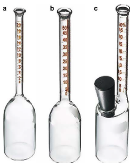
Babcock Milk Test Bottles for Milk (a) Cream (b) Cheese (Paley bottle) (c) Testing (Courtesy of Kimble Glass Co., Vineland, NJ.)
